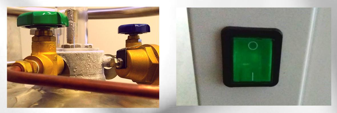
1.Check power connection. Make sure the working pressure is 1,5bar and there is enough nitrogen. 2. Open appropriate valves as specified by nitrogen supplier.
